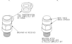
Before putting the unit into operation, it may be necessary to relocate the vent plug for positions other than standard (M1). Substitute the vent plug for the solid plug at the position desired. Install the solid plug in the location the vent plug was removed from. Refer to the following chart for the recommended vent plug locations based on mounting position
