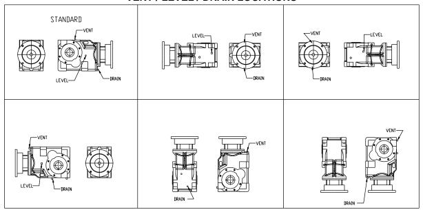
**NOTE:** The unit is filled at the factory with the proper amount of oil for the **STANDARD** mounting position. A level plug is provided for this position only so the unit can be checked for proper oil level prior to installation and start-up. All other mounting positions will require the oil level to be measured out prior to filling the unit based on the values in the table labeled **OIL CAPACITIES** above.
